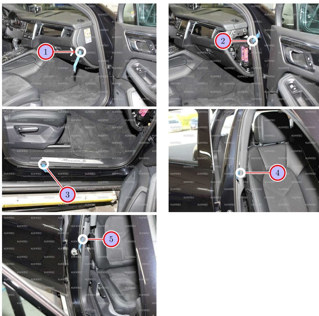
Figure 4: Removing front trim panel passenger's side
